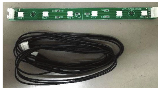
LED lights and linking cable
